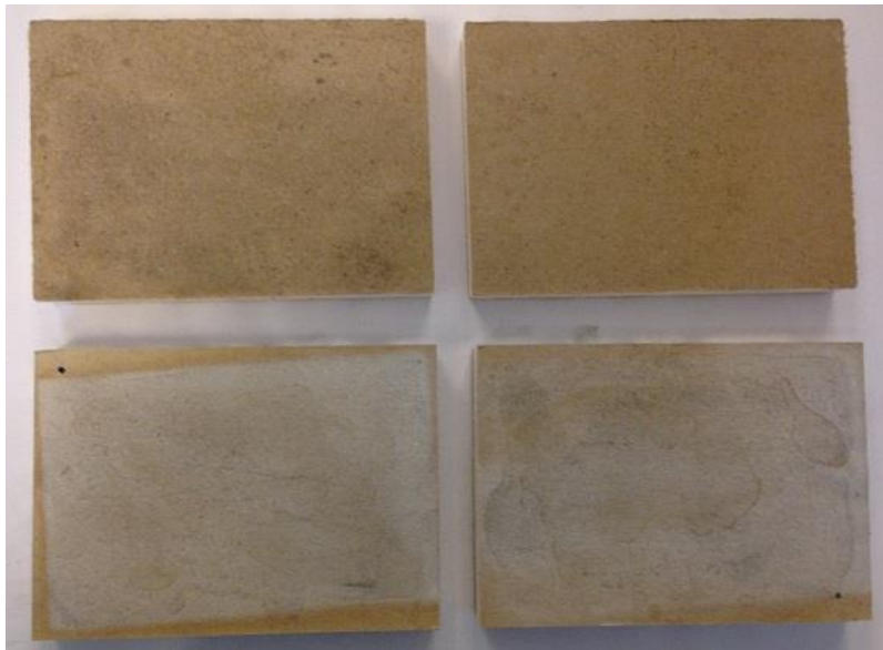
Photo 7. Gypsum boards, growth on surfaces after 7 weeks' exposure
